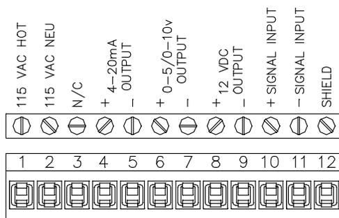
**For +12VDC with Analog Output**
